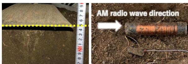
Fig. 3. Photograph of coil antenna sensor embedded in soil
