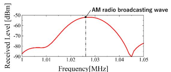
Fig. 2. Measured frequency spectrum of AM radio broadcasting wave by fabricated coil antenna sensor embedded in soil.
