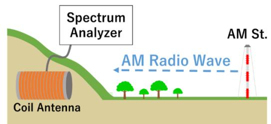
Fig. 1. Overview of monitoring system for water content in soil
