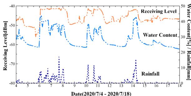
Fig.5. Measured AM radio receiving level (Orange), water content in soil (Blue), and rainfall (Navy blue) in time series.
