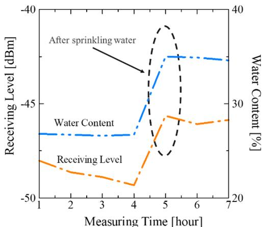
Fig.4. Measured AM radio receiving level (Red) and water content in soil (Blue) versus time.
